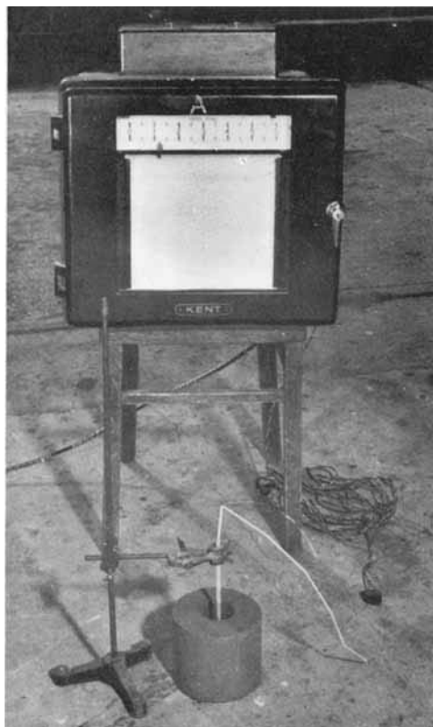
The apparatus for the rapid determination of cooling curves on the foundry floor. A platinum:rhodium-platinum thermocouple measures the temperature of the metal during cooling
