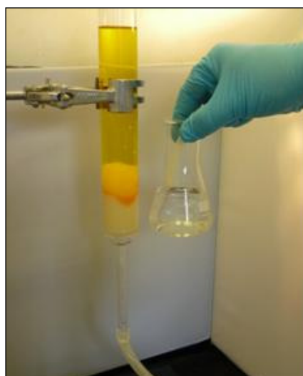
Fig. 2. Smopex ® test column, showing the effective recovery of platinum from a solution of \sim 500 \text{ mg l}^{-1} chloroplatinic acid in aqueous, dilute hydrochloric acid
