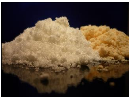
Fig. 1. Examples of some Smopex ® fibres: Smopex ® -102 (foreground) and Smopex ® -112 (background)
