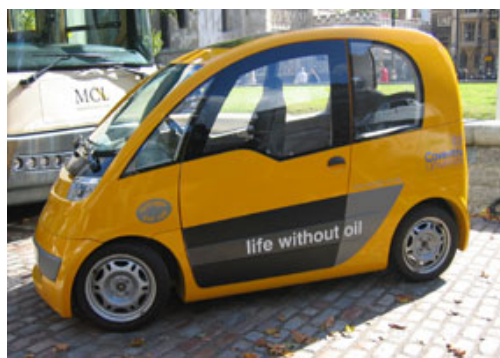
A fuel cell powered Micro Taxi built by Coventry University, U.K.
