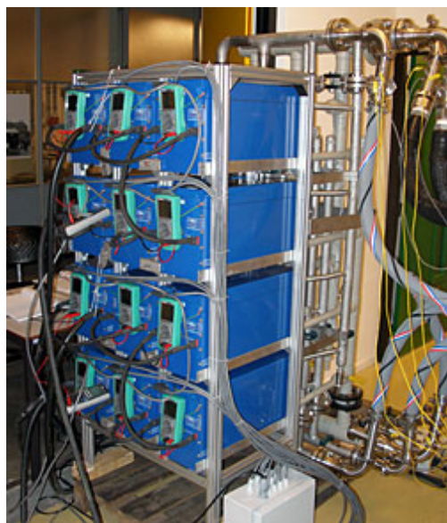
NedStack 50 kW fuel cell module, used in the demonstration project at Chemiepark Delfzijl, The Netherlands (Courtesy of NedStack)
